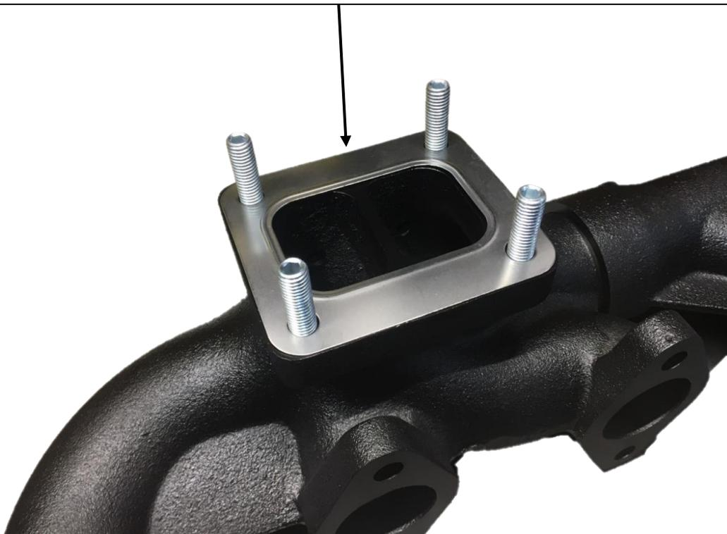
**Step 3:** Secure the T4 turbo flange onto the manifold flange allowing the four **B** studs to pass through the four holes on the turbo flange.
