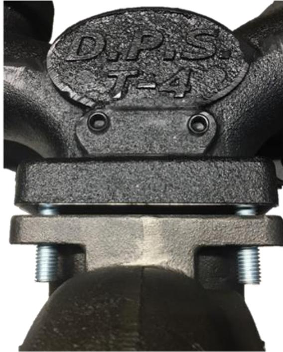
**Step 4:** Thread and tighten four **C** nuts onto the four **D** studs that pass through the back side of the turbo flange. Tighten the nuts to 35 ft-lbs.
